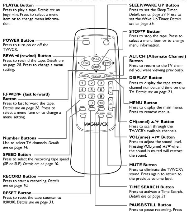
again to resume recording. Details are on page 10. During tape playback, press to freeze the picture (still). Details are on page 28.
